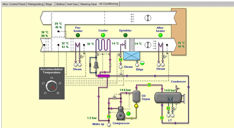
The mimic diagrams present the layout of all vital engine room systems. They include active valves, animated status indicators and tank level gauges.
