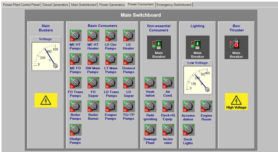
The control panels include very realistic, animated virtual controls like switches, gauges and lamps. The control panels imitate the most important parts of the control room equipment.
