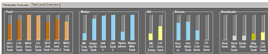
The Tank Level Overview shows the liquid level in the most important tanks from the whole engine room combined into media groups.
