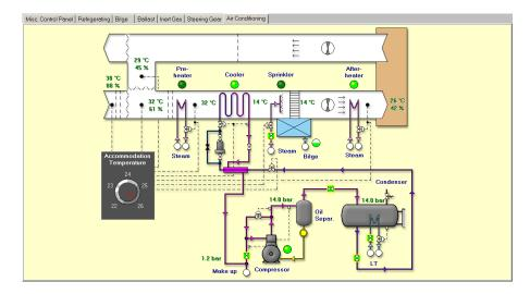
Mimic diagrams present the layout of all vital engine room systems. They include active valves, animated status indicators and tank level gauges.
