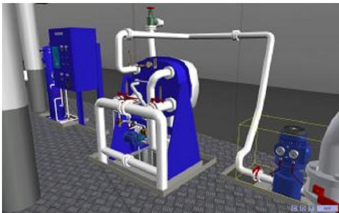
Fig. 10 MED3DH– Fresh water generator installation
