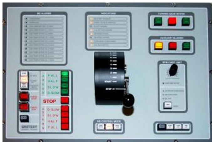
Fig. 23 ERC 4.5 XL Main Engine Control Console lower part.
