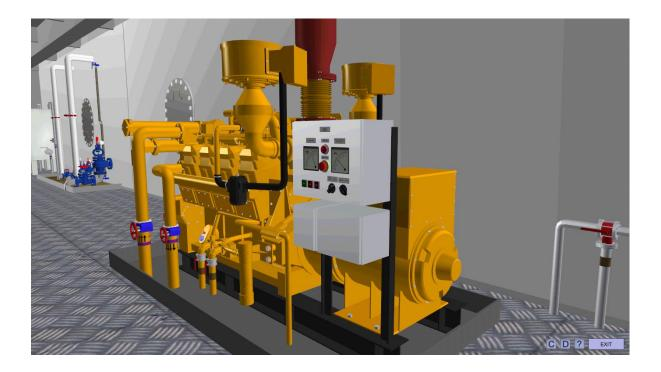
The simulator provides a 3D model of the engine room based on real equipment, and it generates realistic 3D sound which can be heard on two, four or more speakers.
