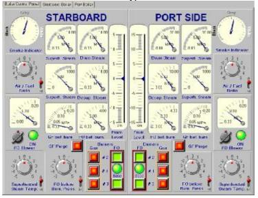
Control panels include very realistic, animated virtual controls like switches, gauges and lamps. The control panels imitate the most important parts of the control room equipment.
