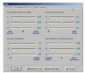
**Evaluation mode** (default): The trainee can freely change the technical state of the engine elements as well as the engine load and operation conditions. This includes the possibility of inspecting the present technical state of the engine elements. This mode can be used for testing the relation between the engine operation conditions or the technical state on one hand, and the engine operation parameters on the other hand.
