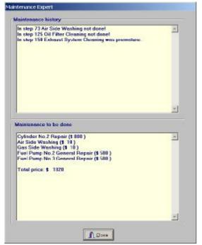
The **Maintenance Expert** can suggest necessary maintenance and evaluate what maintenance was necessary but not done. The upper **History** subwindow shows information about necessary (but not done) and unnecessary maintenance. This information is very useful when working in Run Replay mode. The lower **To Do** window shows all maintenance necessary in the current technical state. This feature is very useful, mainly in the early stages of training.
