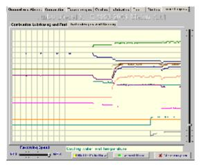
**Time diagram**: The time diagram shows parameter deviation change as a function of a time. This feature is especially useful in Live Run mode.
