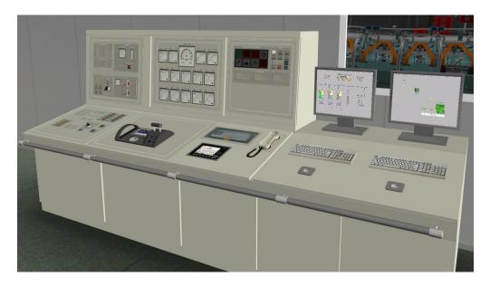
The simulated control room enables remote control of engine room equipment and control panels model the most important elements.
