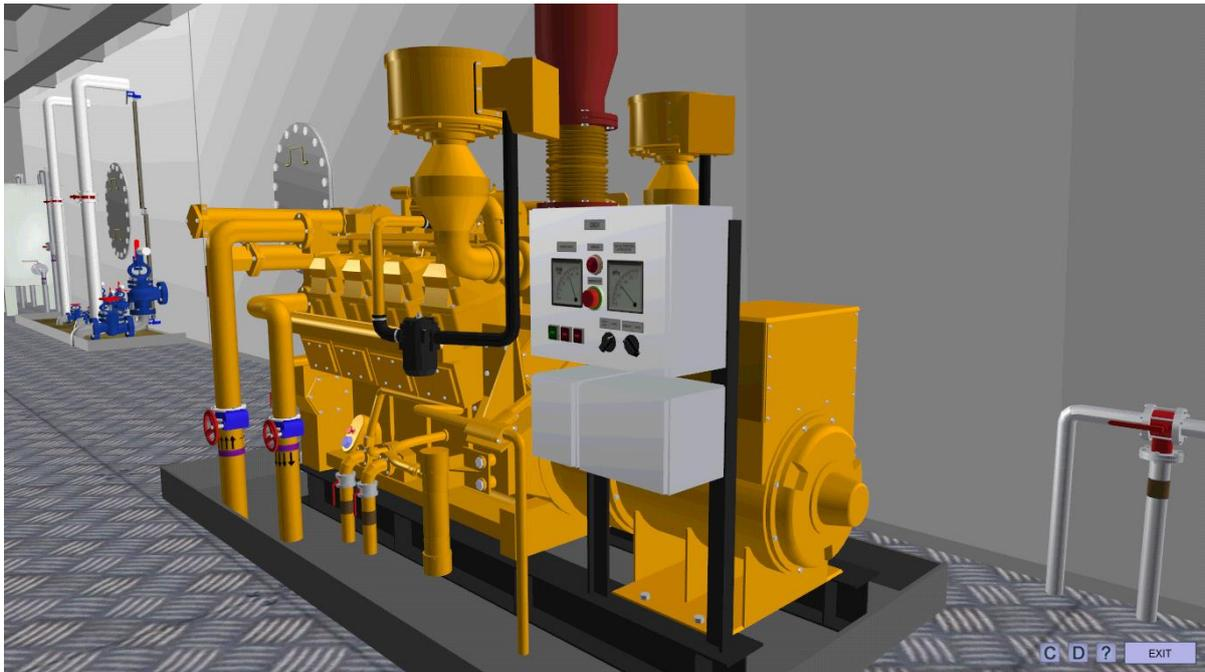
The simulator provides a 3D model of the engine room based on real equipment, and it generates realistic 3D sound which can be heard on two, four or more speakers.
