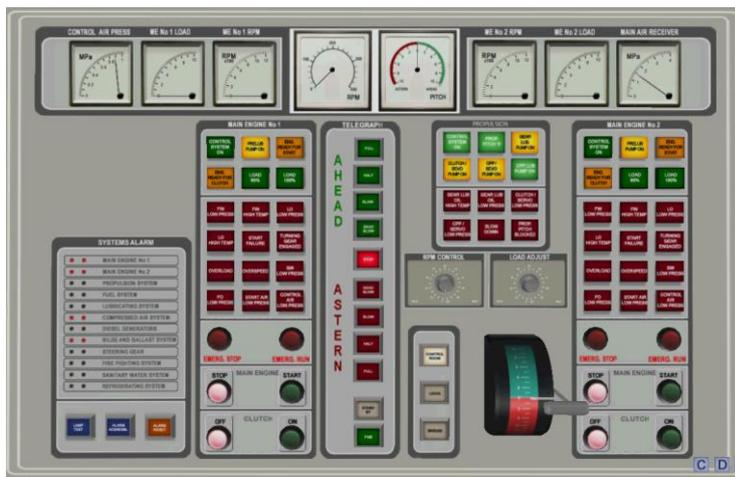
The control panels imitate the most important parts of the control room equipment.
