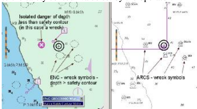
Figure 1 An example of the use of the Isolated Danger symbol on an ENC
